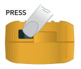
To fit the battery, push the top of the battery into the radio, before pressing it home at the bottom. Ensure that the grey button has locked the battery in place.
